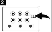
When connected to an external TV, slide the CDG/CAMERA switch to the CAMERA position to see the image from the camera on the external TV.
